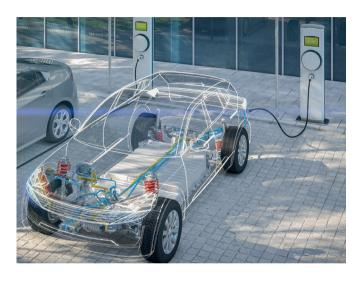
**Power electronics controller:** This unit manages the flow of electrical energy provided by the traction battery, controlling the speed of the electric traction motor and the torque that it produces.
